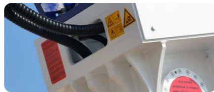
▼ Housing with hydraulic hose protection.
