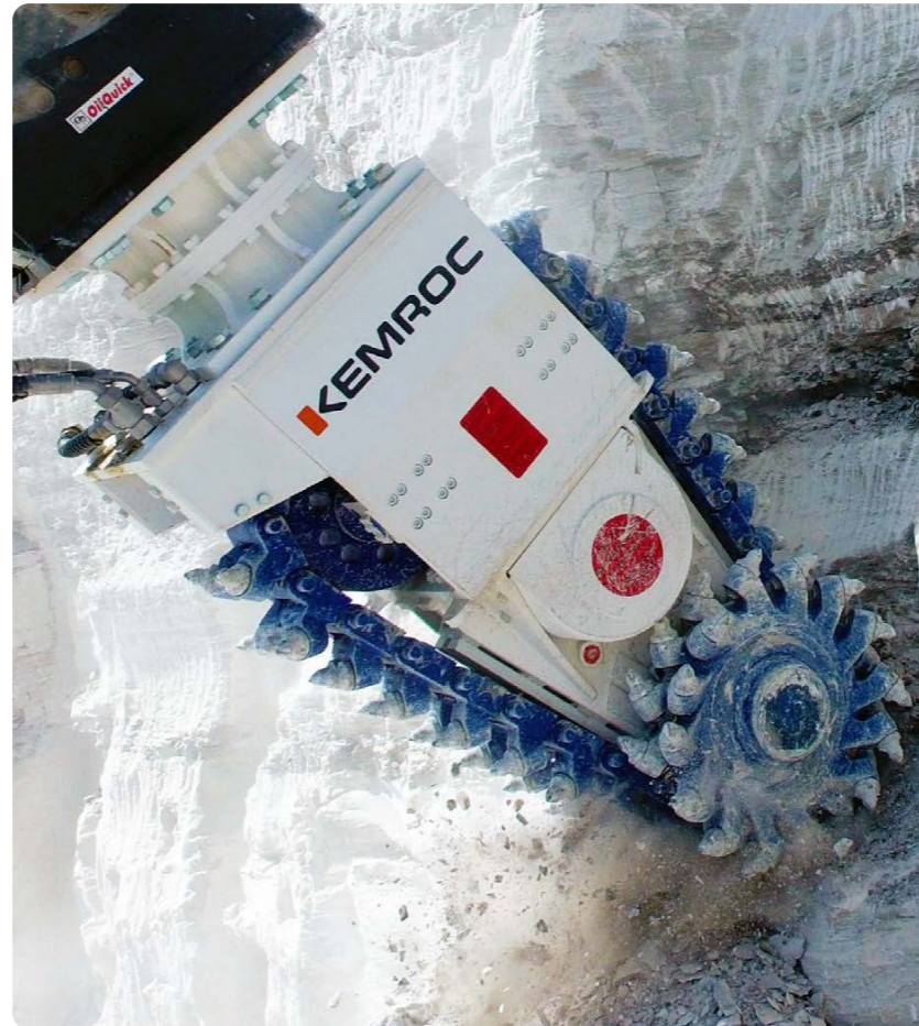
▲ Mining gypsum with an EK 100.
