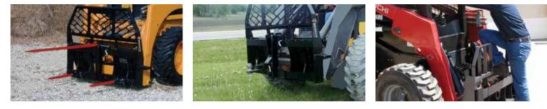
Optional features include an Auger Mount, Bale Spear, & 2" Trailer Receiver Hitch. An additional frame option includes 2" drop height for loaders with oversized tires or tracks over tires is available.
