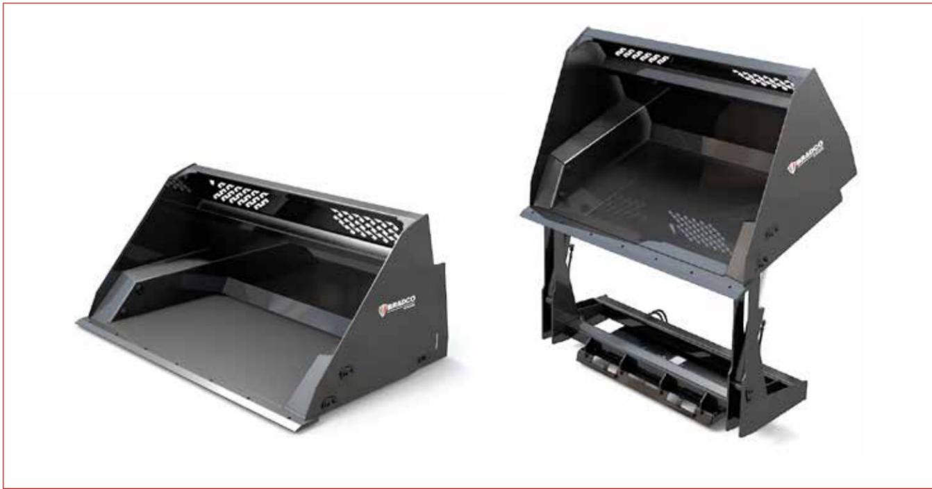
The Bradco® High-Dump line of buckets allow users to increase the dumping height of their machine by 74 inches and load material into trucks, feed bins and reach other landing heights previously not obtainable with a standard bucket. This light material high-dump bucket exceeds all competitive units by offering increased capacities, cushioned hydraulics, 114° of roll out and the most robust design in the industry. These features translate to higher productivity and faster cycle times.
