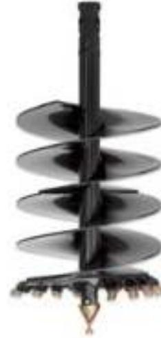
These Augers are made for difficult ground conditions, compacted soils, heavy clay, frozen ground and fracturable rock. The HDC Augers feature heavy duty cast steel boring head, hardened drive-in gage (outside) and wisdom (inside) teeth. Equipped with hardened fishtail point and heavy-duty, double flighting.
