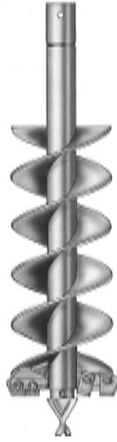
These Augers are made for light to moderate ground conditions. The HDF augers feature a fabricated boring head with hardened bolt-on gage (outside) and wisdom (inside) teeth, as well as a hardened fishtail point. These augers also are equipped with heavy-duty double flighting.
