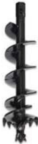
These Augers are made for solid, fracturable rock, frozen ground, asphalt and compacted soils. These rock augers feature bullet style teeth and a fabricated boring head, as well as heavy-duty single flighting. This auger comes in 2" hexagon collar only and is available in 4' length. The auger has a .75" thick bottom flight and a hardface outer edge.
