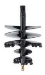
These Augers are made for tree and shrub planting. The HTF augers have a 2" diameter design with a fabricated boring head and hardened bold-on gauge (outside) and wisdom (inside) teeth. Augers also come equipped with a hardened fishtail point and heavy-duty double flighting.
