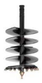
These Augers are made for difficult ground conditions, compacted soils, heavy clay, frozen ground and fracturable rock. The HDC Augers feature heavy duty cast steel boring head, hardened drive-in gage (outside) and wisdom (inside) teeth. Equipped with hardened fishtail point and heavy-duty, double flighting.
