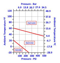
Remember: Insufficient lubrication or incorrect lubrication grades may result in damage being caused to the hammer and it's components. Hydraulic oils, engine oils, gear oils and diesel are not recommended for lubricating DTH hammers.
