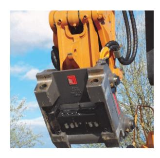
OilQuick is an automatic quick coupler system for excavators, which allows hydraulic work tools to be connected and disconnected from the drivers cab.
