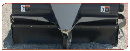
A double drape system seals the sweeping chamber to the ground
