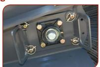
After resting the sweeper on the ground, remove the pins from motor and bearing mounts
