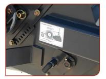
A simple tool-less adjustment knob allows you to accommodate brush wear and still maintain increased bucket capacity
