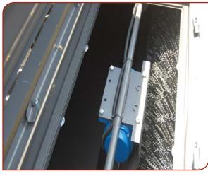
12 volt shaker dislodges loose debris from the filter media directly into the hopper
