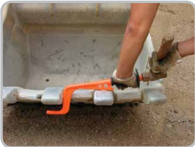
1. Input small pin into tooth-hole and punch
